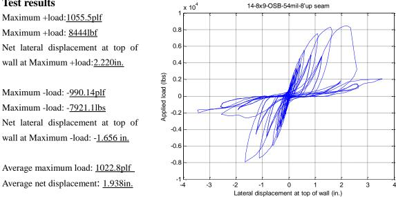
Observed Failure Mode: Failure occur at bottom fasteners pull through OSB, fasteners at chord studs up to 3'pull through and several wood bearing failures observed.
