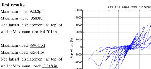
Average maximum load: 905.5plf Average net displacement: 3.559in. -3000 -4000 -5000 -4 -3 -2 0 2 3 4 -1 Lateral displacement at top of wall (in.)
