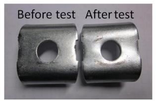
Figure 10 Deformation of hold-down (view from bottom, test 12 shown)
