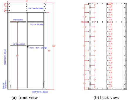
Figure 6 Shear wall specimen drawing (details are the same for 8 ft wide shear walls)
