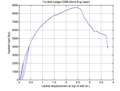
**Observed Failure Mode:** Failure occurred at vertical seam with wood bearing failure and fasteners pulled through OSB. .
