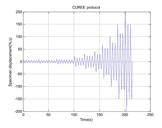
Figure 5 CUREE loading history as realized in a test
