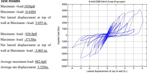
Observed Failure Mode: Fasteners at vertical seam (without additional stud ) pulled through OSB.
