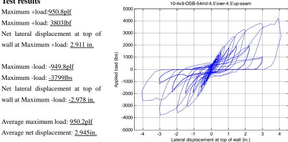
**Observed Failure Mode:** Fasteners at vertical seam location (south bottom part of OSB) pulled through OSB.
