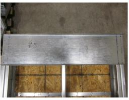
(a) Ledger attached to top of shear wall
