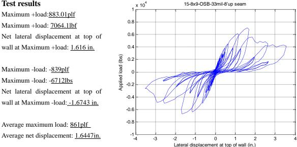
Observed Failure Mode: Failure occurred at vertical and horizontal seam with fastener tilted and pulled through OSB.
