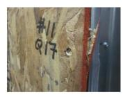
(b) wood bearing failure (WB)
