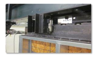
Figure 3 Close-up of out-of-plane support and WT shape
