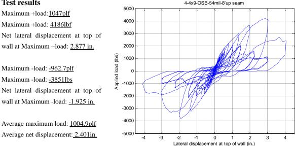
**Observed Failure Mode:** Fasteners in the seam location pulled through OSB.
