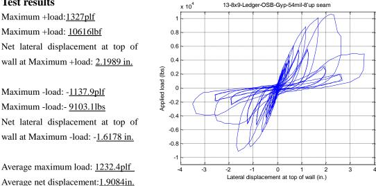
**Observed Failure Mode:** Failure occurred at OSB bottom and gypsum board. Fasteners at gypsum board enlarge holes, major of fasteners pull through board. South side gypsum board already separated from the frame. OSB side, bottom fasteners at bottom and chord stud up to2' pulled through OSB.
